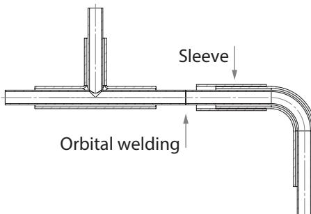
1. Assemble the sleeve over the inner tube.
