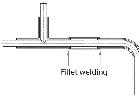
1. Slide the sleeve over the inner tube to close the gap between the outer jackets.
