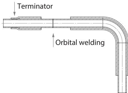
1. Assemble the terminator over the inner tube.
